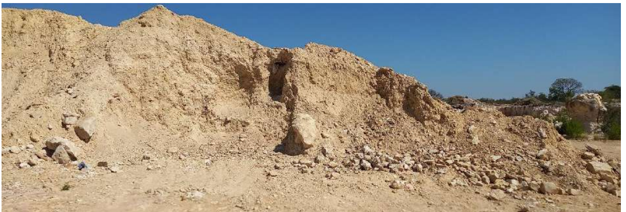
Figure 5: A stockpile of G7 material in the borrow pit
