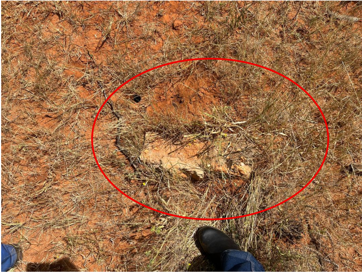
Figure 7: Partially exposed rock fragment observed within the project area, indicating underlying bedrock beneath predominantly surficial deposits.
