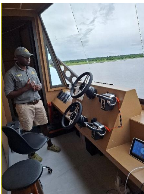
Figure 5: The wheelhouse for the PV at the bow of the boat with a 180-degree view.
