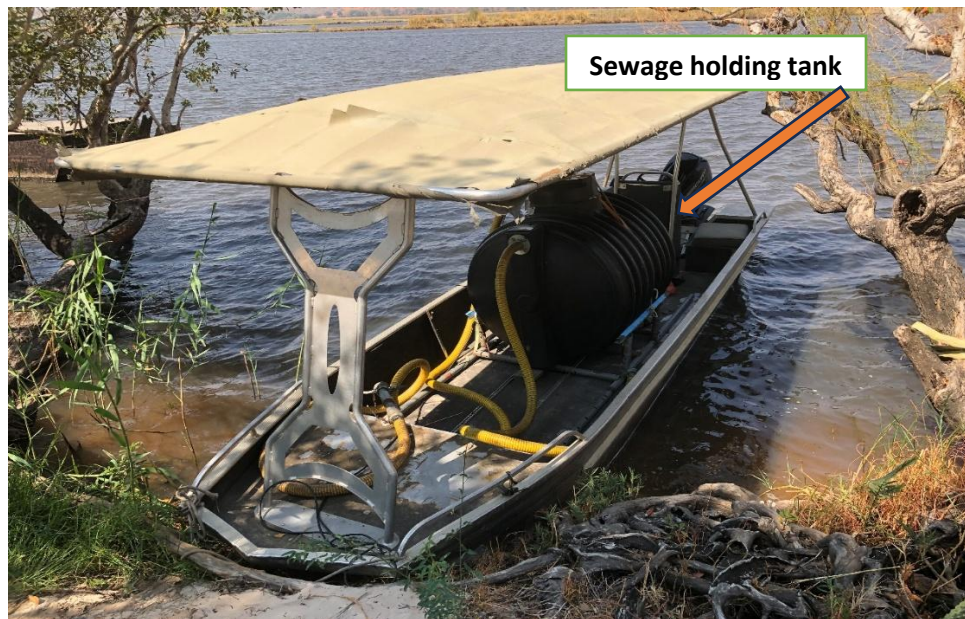
Figure 10: Boat used to transport sewage from the PV to ZEL sewage treatment system
