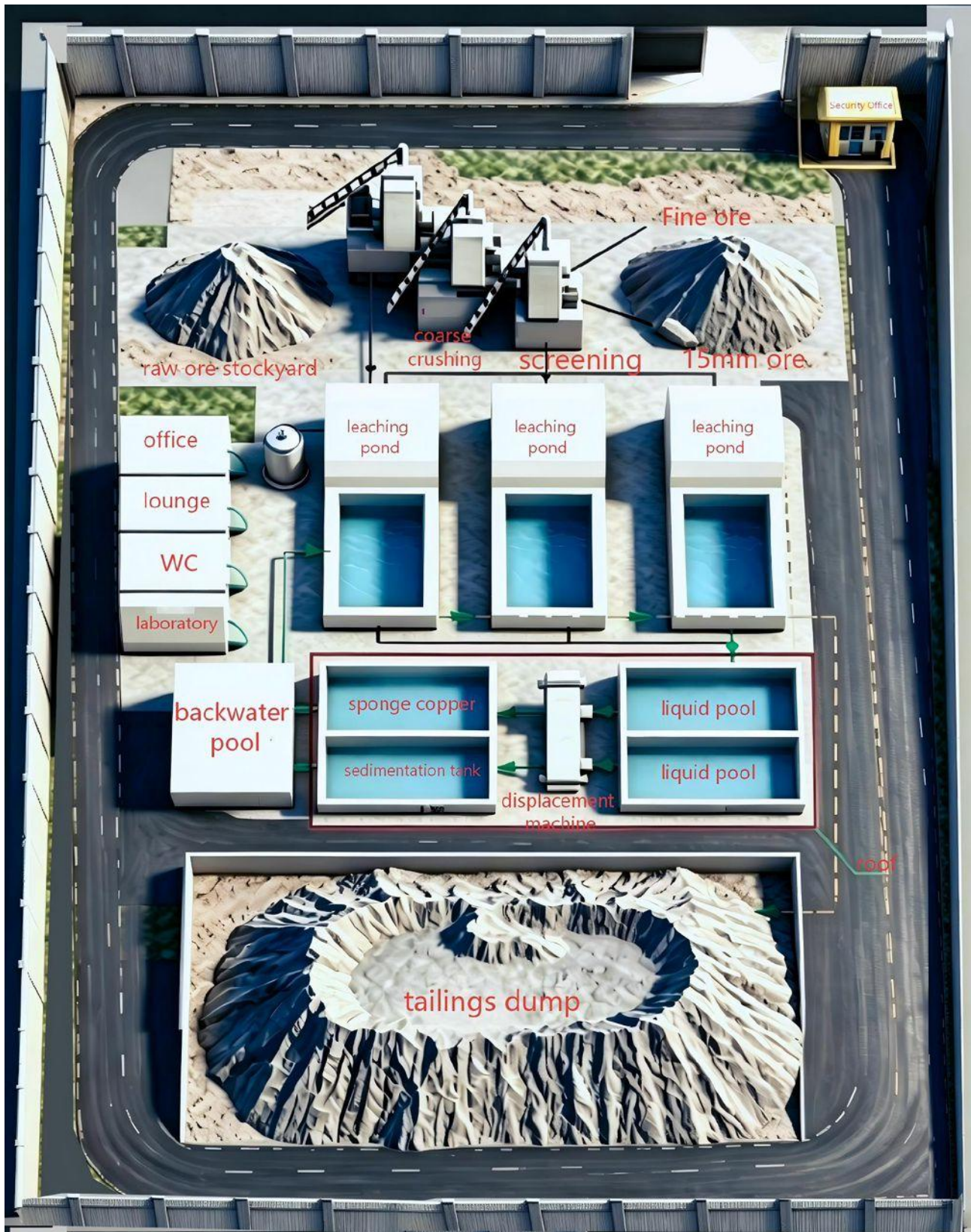
Figure 1: Plant Design and Copper Ore Processing Flow
