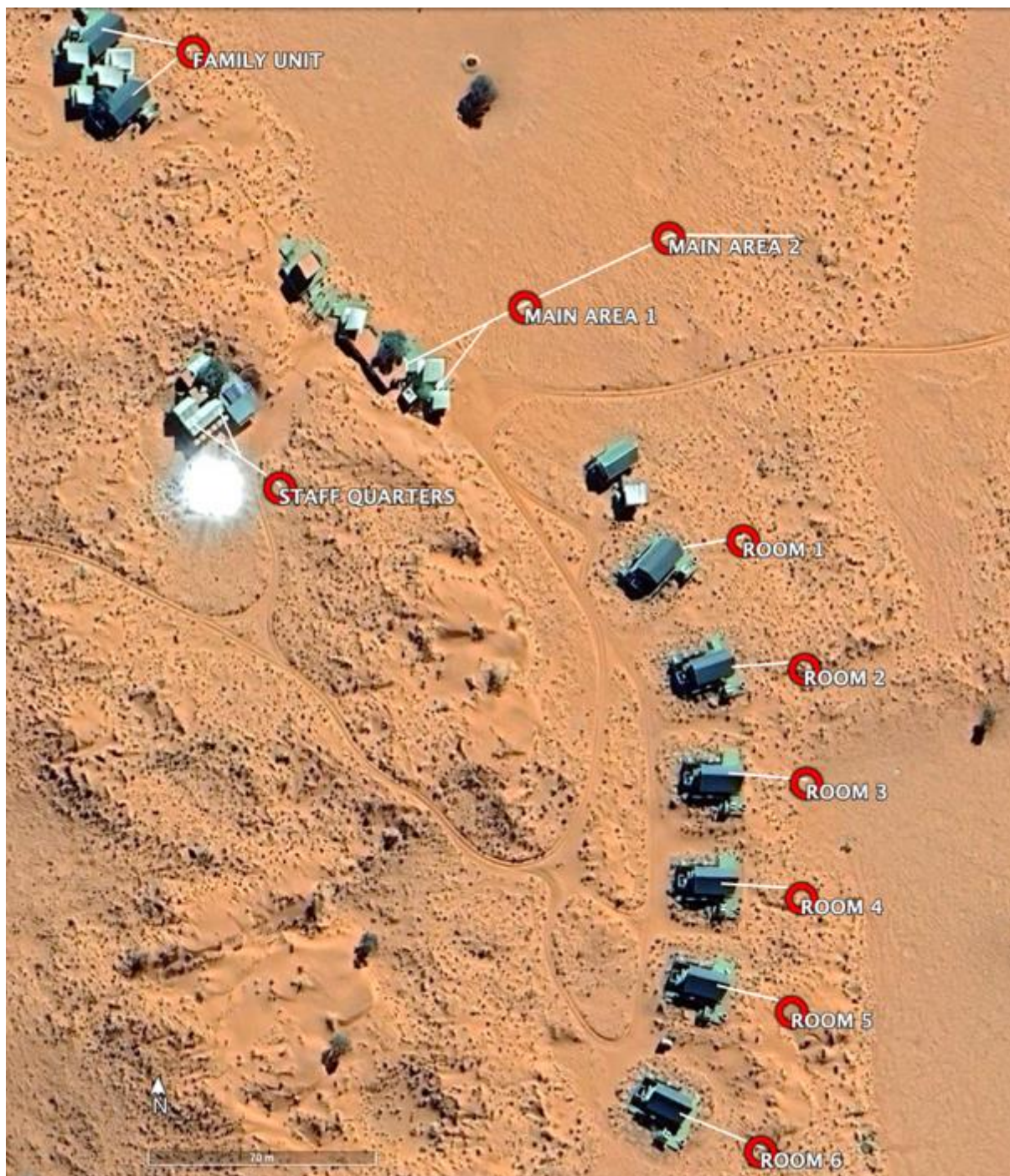
Figure 2. Infrastructure at Dunes Camp. The red circles represent septic tanks.
