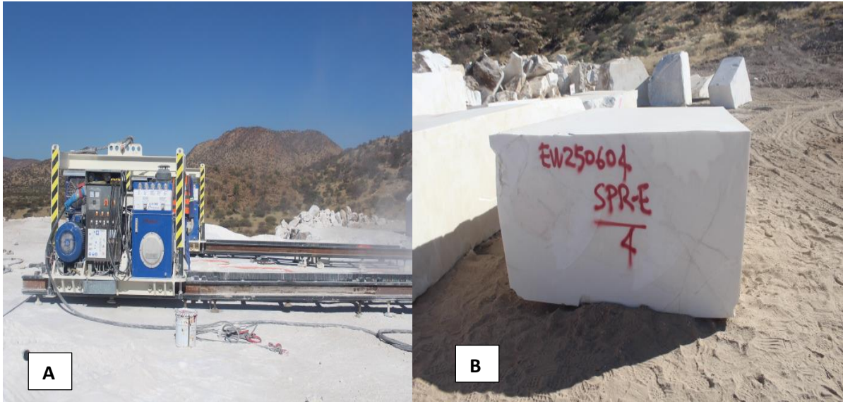
Figure 3: The marble block cutting machine (A) and a block of white marble (B) that will be mined at ML 270
