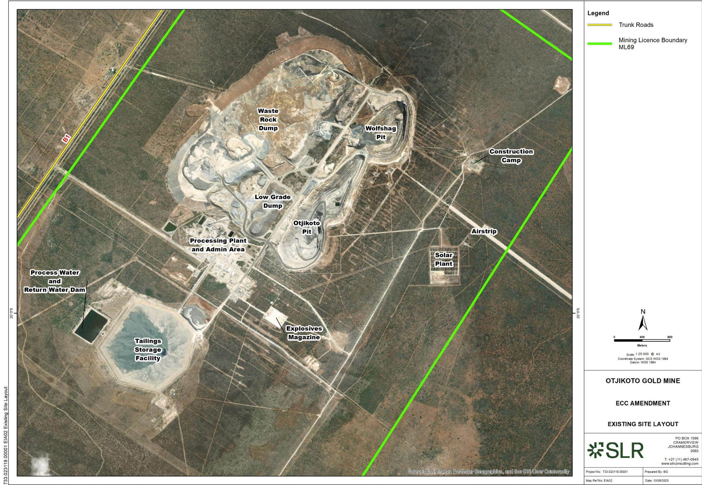
Figure 2-1: Existing Infrastructure Layout
