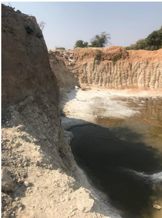
Figure 4: Reason why mining restricted to 4m deep or 1m above ground water table
