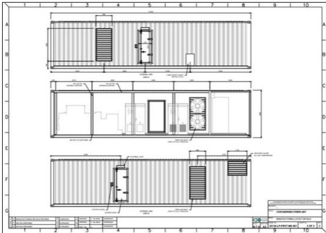
Figure 8: Genset container and layout (2)
