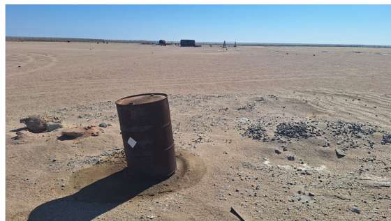
Photo 3-6 Leaking fuel storage for training
