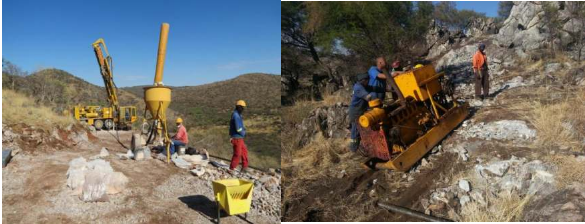
Figure 5. A truck mounted RC drill rig and a skid mounted drill rig (illustration only)
