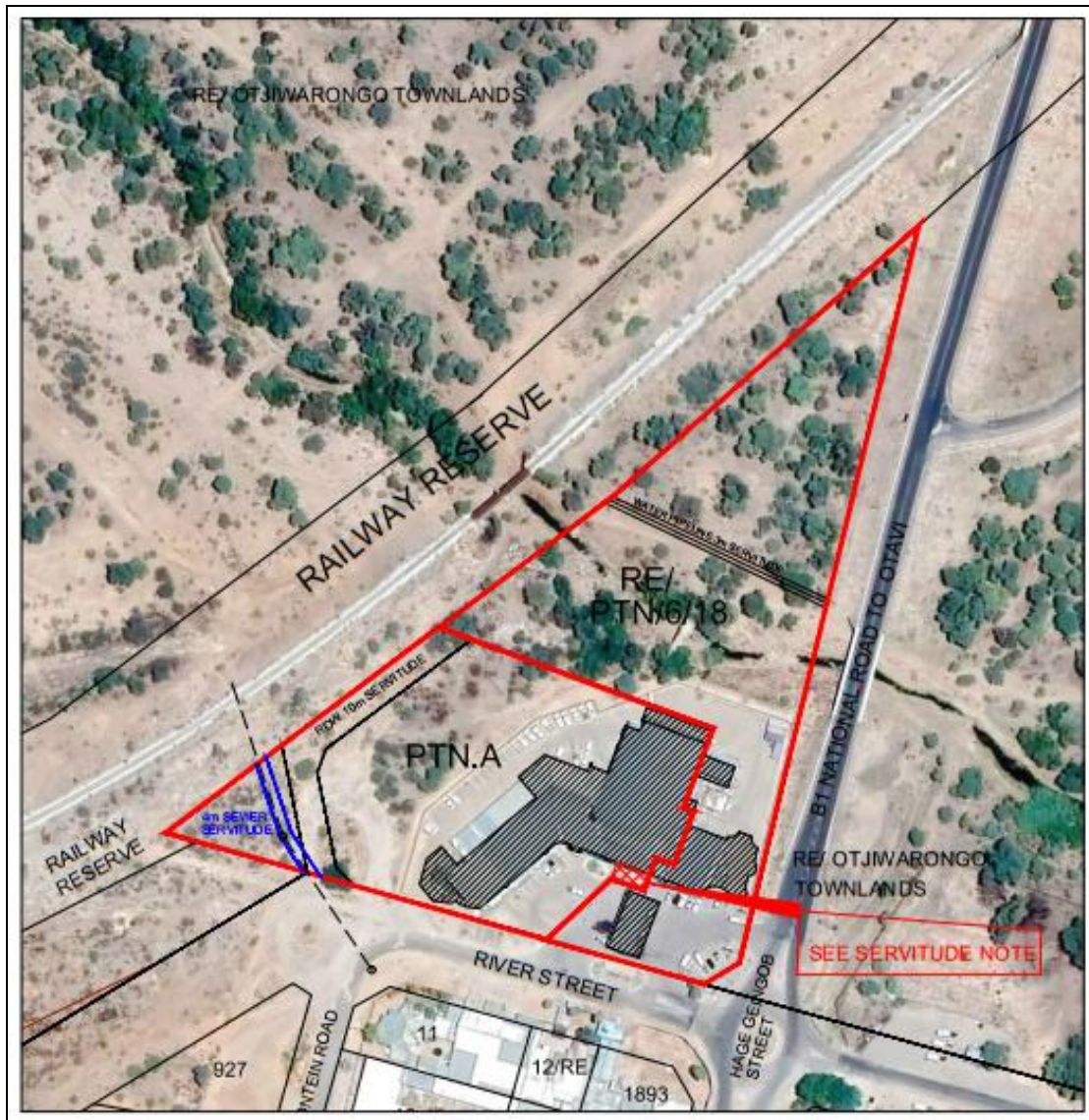
Figure 8: Right of Way servitude along the northwestern boundary
