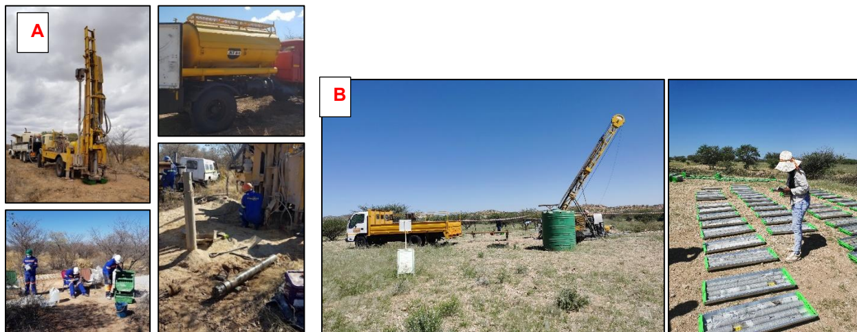
Figure 2-4: A-typical drill rig on an EPL (Resilient Environmental Solutions, 2019), B- drill rig on active EPL precious metals exploration site visited by the Author in Erongo Region (photo by Author, 2022)
