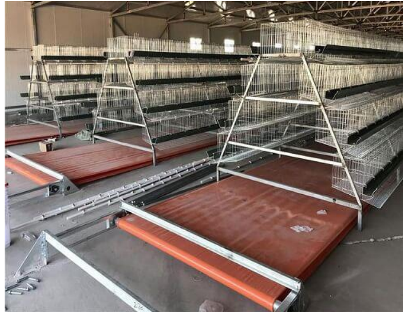
Figure 10: A-Type Cage with Automatic Manure Cleaner Illustration
