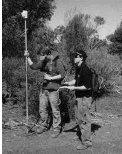
FIGURE 7. ILLUSTRATIVE IMAGE OF A GROUND-BASED GEOPHYSICAL SURVEY WITH MAGNETOMETER (PHOTO TAKEN FROM: HTTPS://IRSL.SS.NCU.EDU.TW/MEDIA/COURSE/CI/SIO_9.PDF )
