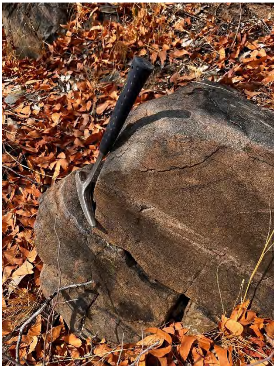
Figure 6-3: Grey biotite schist outcrop, medium grained texture and translucent quartz veins sub-parallel to the country rock.
