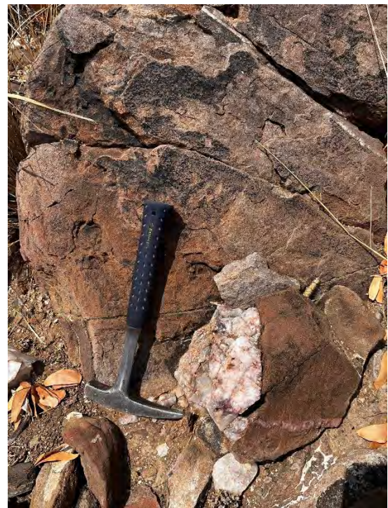
Figure 6-3: Grey biotite schist outcrop, medium grained texture and translucent quartz veins sub-parallel to the country rock.
