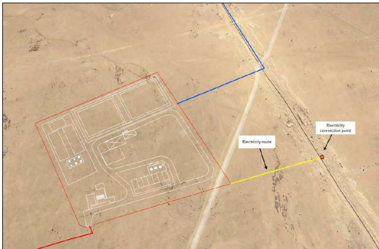
Figure 12: Electricity Supply Route
