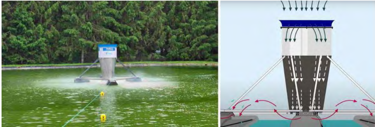
Figure 9: Floating surface evaporator unit for enhanced evaporation
